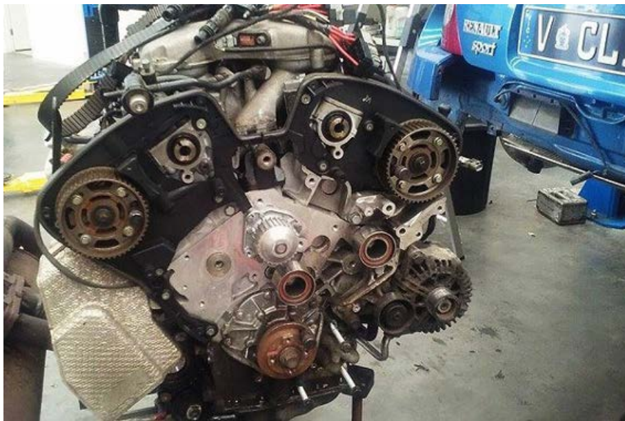
Timing belt change = engine out job
